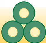
3-Strand Spun and Filament Polyester Jacket Fibers Covering Polyolefin Core Fibers.
